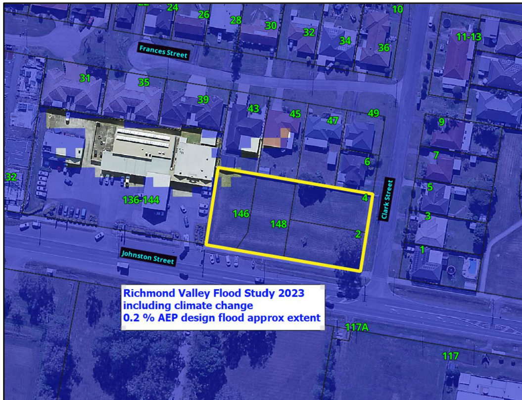
Figure 22: 0.2% AEP design flood inc. CC (extract Richmond Valley Flood Study 2023)
