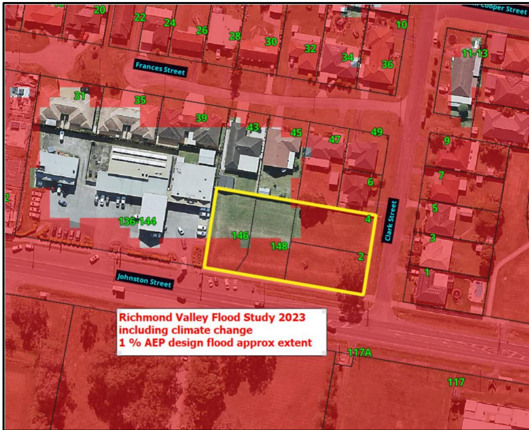
Figure 21: 1% AEP design flood inc. CC (extract Richmond Valley Flood Study 2023)
